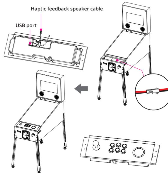
**Step 4.** Repeat Step 1 in reverse to re-assemble the machine. Place the left and right side panels back to their original positions by the main display and secure them with the 10 screws. Once both left and right side panels are reattached, replace the front panel and fasten with the 3 screws.
