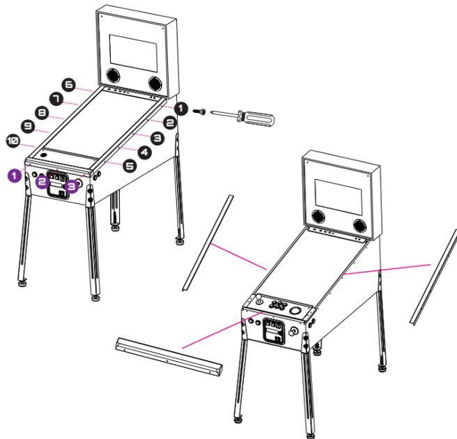
**Step 2.** Remove the screws and lift up the original control top. Carefully detach the D-pad connecting cable and haptic feedback speaker cable. Remove the screws holding the USB cable.
