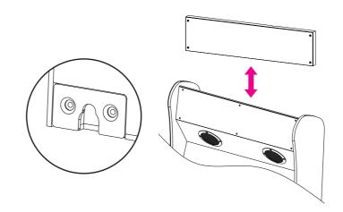
Step 6. Remove the 6 screws from the back panel.
