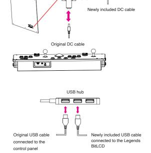
Step 11. (Legends Ultimate 1.1 or newer owners skip to Step 12.) Connect the USB cable to the right-most USB port of the Control Panel.
