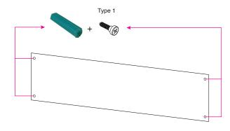
Step 2. Slide the BitLCD slowly downward on the exposed screw heads until it is secured in place.
