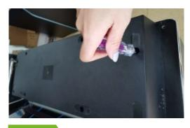
**Step 12** Put the control top cover back and fasten the screws.
