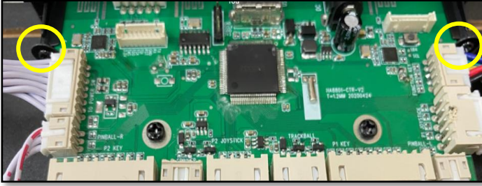
7. Unscrew both screws on the side to remove the CTR board.
