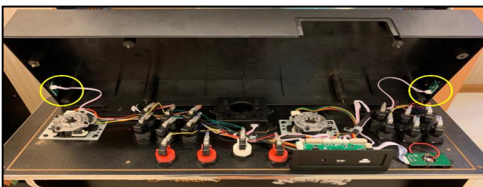
13. Attach the Pinball cables from step 3.
