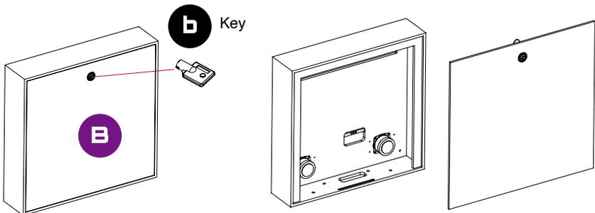
Step 3. Take out the backglass and the included [b] key. Use the key to open up the rear panel on the backglass.
