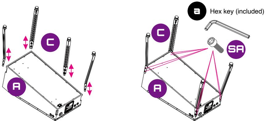
Step 1. Take out the playfield, legs, and 8 [SA] screws. Put the playfield upside down on a soft surface. Attach the legs to the main cabinet and insert 8 [SA] screws to the matching holes with [a] hex key.
