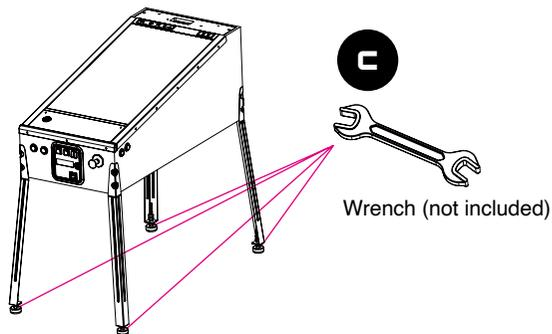
Step 2. Position the playfield upright. Use the [c] wrench to adjust the height of the playfield to your liking. Tighten the base screws when set.
