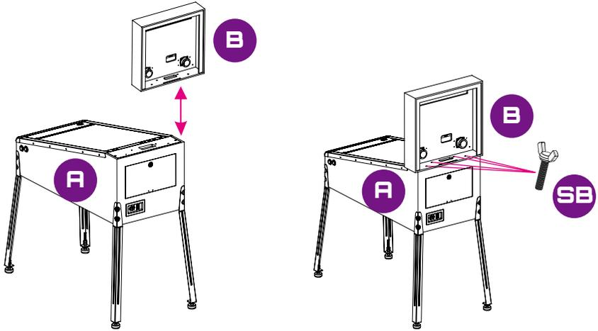
Step 4. Attach the backglass to the top of the playfield. Tightly insert 4 [SB] screws to the matching holes. Securely connect the cords to the matching slots.
