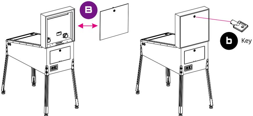
Step 5. Attach the back cover of the backglass and tighten it with the included [b] key.
