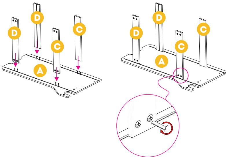
Step 3. Lay [A] aside and take out one [C]. Insert [C] into [A]. Please note the sides with holes face outwards. Use a straight head screwdriver to rotate [S2] with mark "+" to tighten. Repeat process for the rest of [C] and [D].
