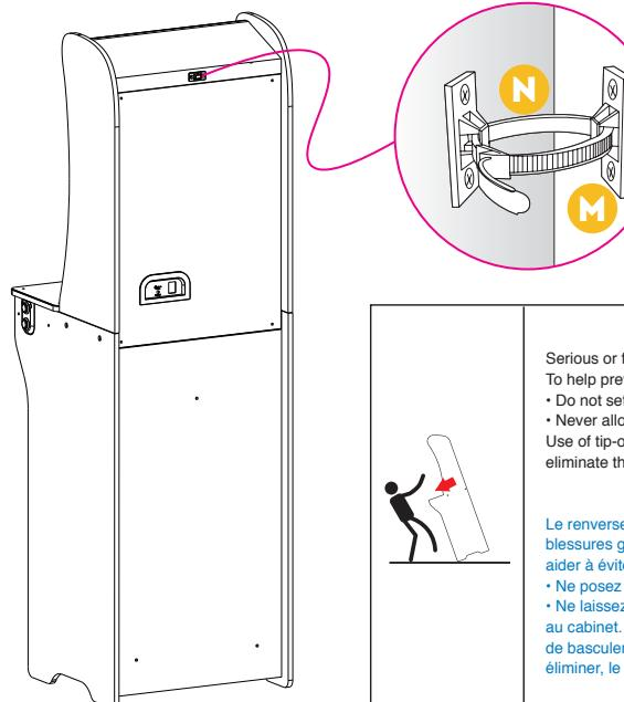
Step 15. Tighten [S7] on the bracket [M] against the wall.
