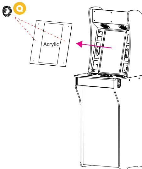
Step 2. Use the suction cup [Q] to remove the acrylic panel.
