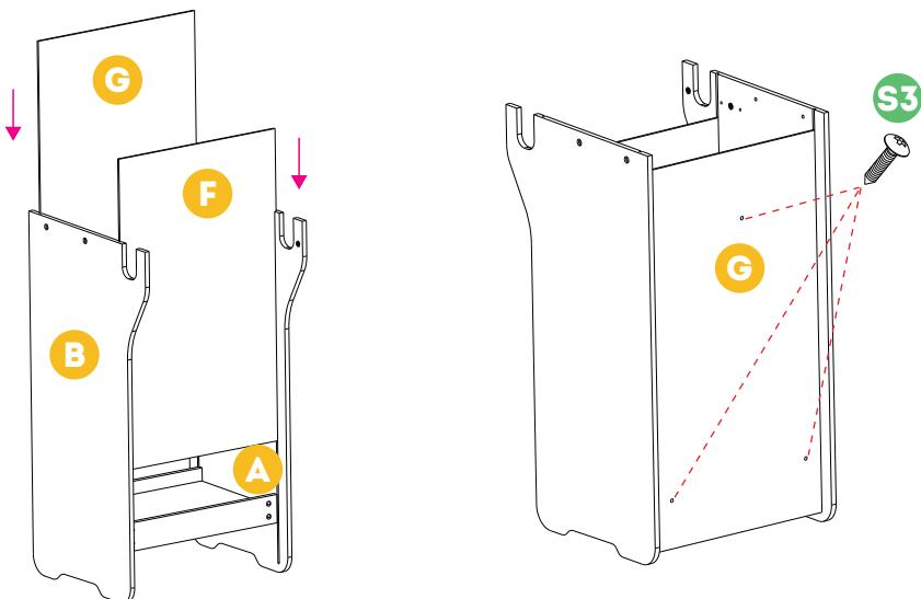
Step 6. Slide [G] and [F] into the tracks of [A] and [B].
