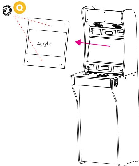
Step 2. Use the suction cup [Q] to remove the acrylic panel.
