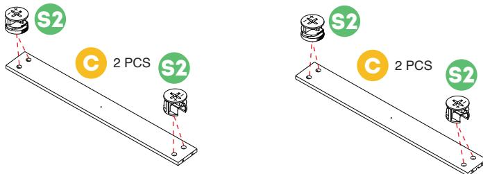
Step 2. Insert 16 [S2] screws to the matching holes on the pairs of [C] and [D]. Please note the side with the slots faces outwards.
