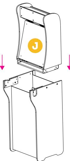
Step 9. Attach bar top [J] to the bottom part of the cabinet.
