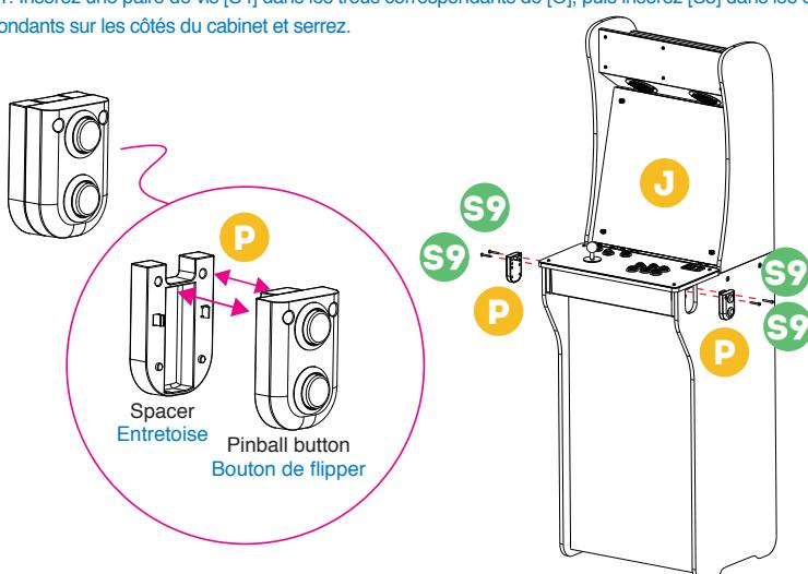
Step 12. Remove Spacer from [P] and install the pinball buttons on both sides of the cabinet, then insert [S9] screws into the matching holes on the sides of the cabinet and tighten.
