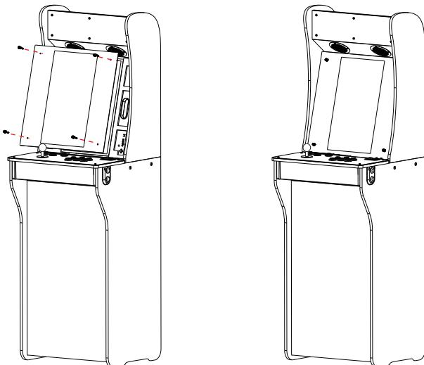
Step 4. Insert 4 thumb screws into the matching holes and tighten.
