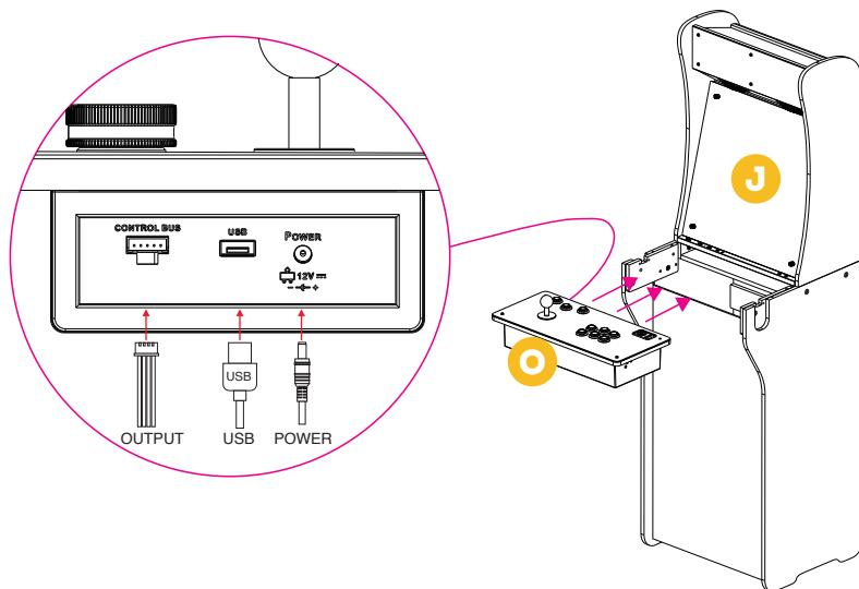
Step 10. Connect the cables to the matching slots on the control panel [O]. Please make sure the slots are aligned. Insert [O] into the cabinet.
