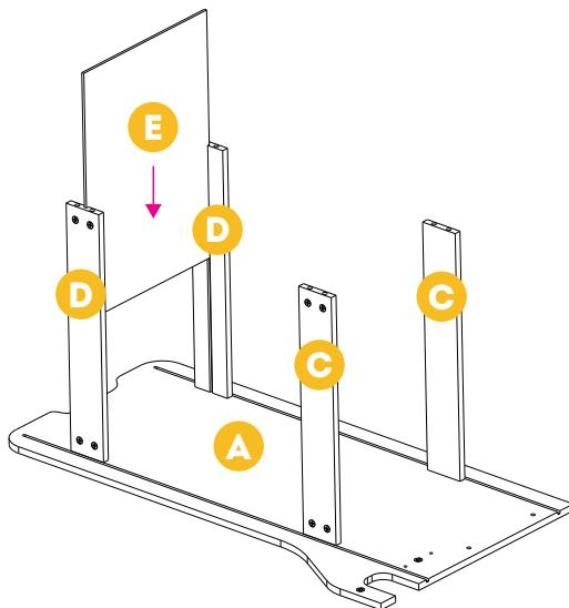
Step 4. Slide [E] into the tracks of the pair of [D].
