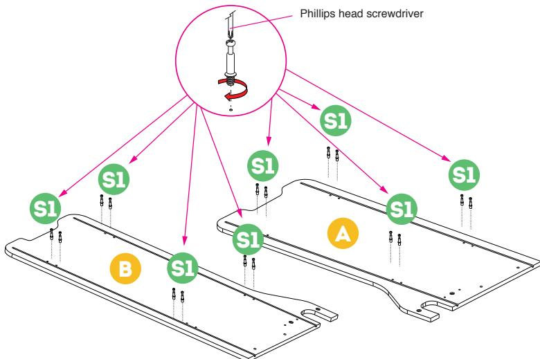
Step 1. Insert the 16 [S1] screws to the matching holes on [A] and [B] on both panels with a Phillips head screwdriver. Please insert and make sure to tighten perpendicular to board (redo this step as needed). Do not use excessive force or you risk breaking the panels.
