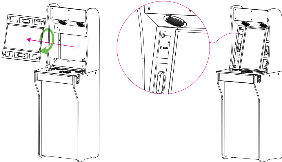
Step 3. Remove the monitor from the machine. Turn the display clockwise, then put the monitor back in the machine.
