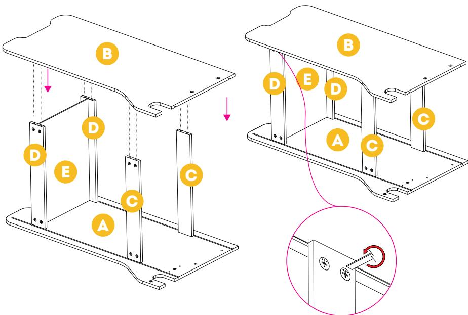
Step 5. Insert [B] to the matching holes on [C] and [D]. Use a straight head screwdriver to rotate the 8 [S2] with mark "+" to tighten.
