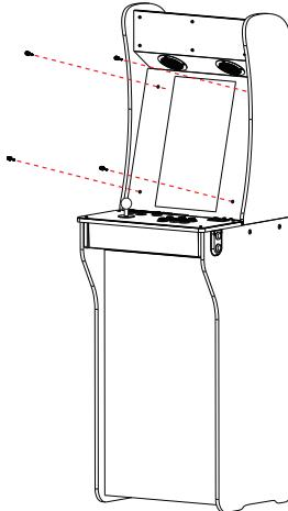
Step 1: Remove the 4 thumb screws from the acrylic panel.
