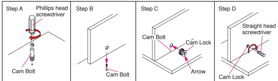
Step A. Use Phillips head screwdriver to fasten the cam bolt onto the panel. To avoid insufficient length to connect the cam lock, please do not overtighten it.
