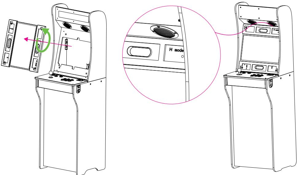
Step 3. Remove the monitor from the machine. Turn the display counterclockwise, then put the monitor back in the machine.
