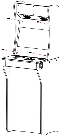
Step 1: Remove the 4 thumb screws from the acrylic panel.
