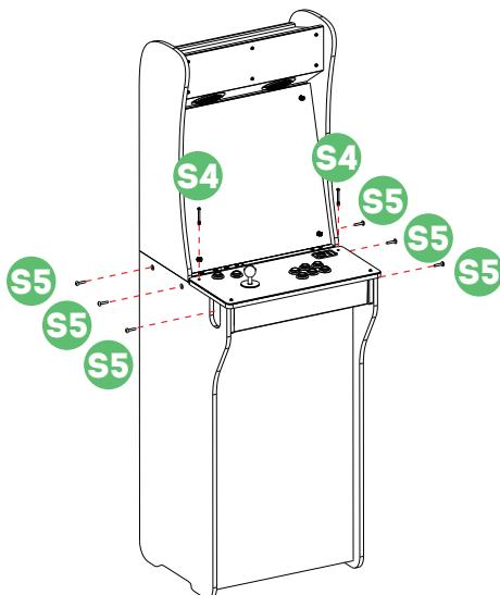
Step 11. Insert a pair of [S4] screws into the matching holes on [O], then insert [S5] to the 6 matching holes on the sides of the cabinet and tighten.
