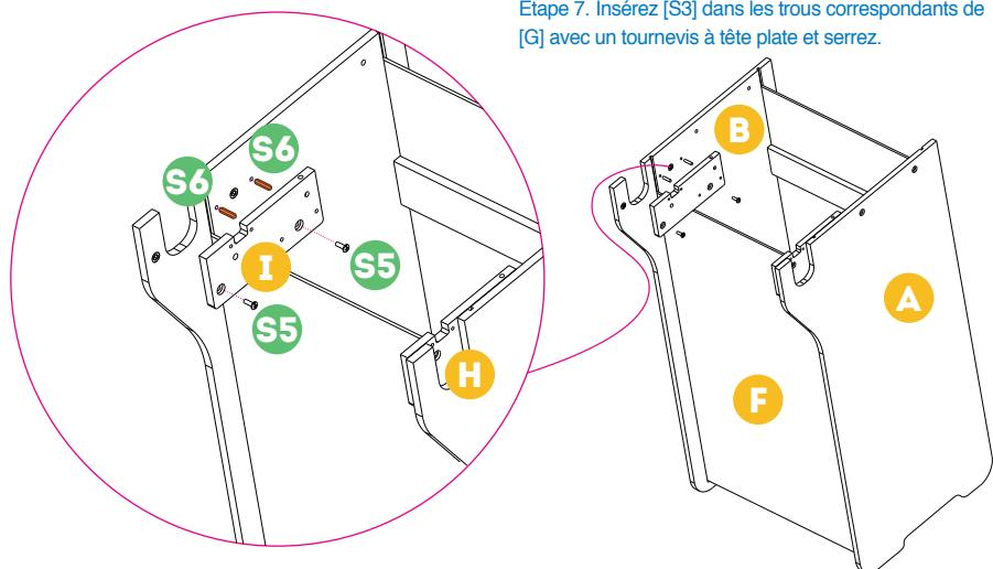
Step 8. Insert the 4 wood dowels [S6] into the [B] panel and install [I] to [B]. Insert 2 screws [S5] into the matching holes on [I] and tighten. Attach [H] to [A] panel in the same manner.
