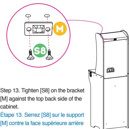
Step 13. Tighten [S8] on the bracket [M] against the top back side of the cabinet.
