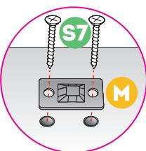
Step 16. Fasten the cable tie [N] to connect both brackets [M] to keep the cabinet from tipping over.
